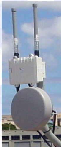
QnodeJr™ equipped with 5.8 Ghz backhaul and 2.4 Ghz diversity radios (photo courtesy Keener Technologies, Inc.)
