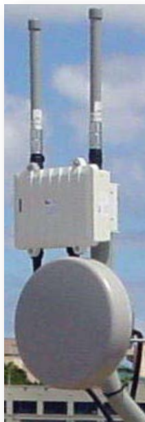
PICTURED Qnode™ equipped with 5.8 GHz backhaul and 2.4 GHz diversity radios (photo courtesy Keener Technologies, Inc.)
