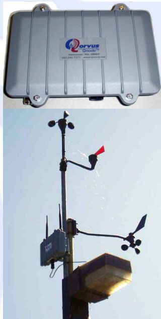
QnodeJr™ equipped with diversity 2.4 Ghz radio does double-duty for weather-data backhaul and internet service to Columbia River barge traffic (photo courtesy Stevenson Wifi Inc.)
